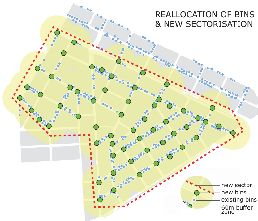
Fig. 5. Reallocation of waste collection bins in the new sector
