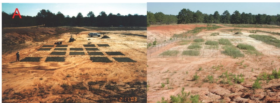
Fig. 2. Borrow Pit field sites on Fort Benning Military Reservation, GA; A) initial application of Fluff, B) plant growth after 2 years.
